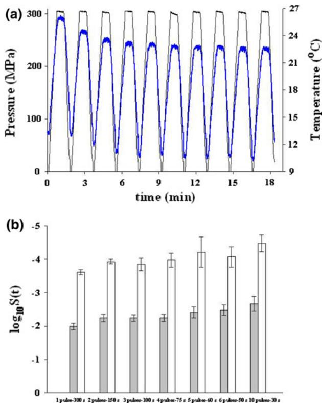
**Fig. 2** a Pressure (upper line) and temperature (lower line) profiles of multi-pulsed HHP (300 MPa) treatment with holding time (30 s  $\times$  10 pulses). b Levels of inactivation of *E. coli* up to 10 pulses with holding time (total holding time = 300 s) in non-selective (grey) and selective (white) media. Error bars represent 95 % confidence intervals
