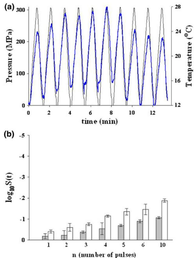
**Fig. 1** a Pressure (upper line) and temperature (lower line) profiles of multi-pulsed HHP treatment (300 MPa) with no holding time (pulse number ranged from 1 to 10). b Levels of inactivation of *E. coli* in non-selective (grey) and selective (white) media. Error bars represent 95 % confidence intervals
